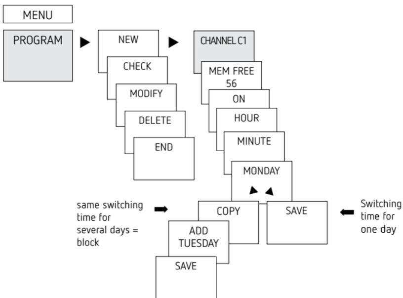
① A switching time always consists of a start time and an end time
